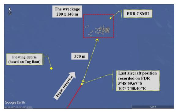
Figure 8: The wreckage distribution
