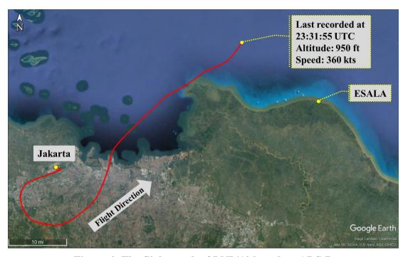
Figure 4: The flight track of LNI610 based on ADS-B
