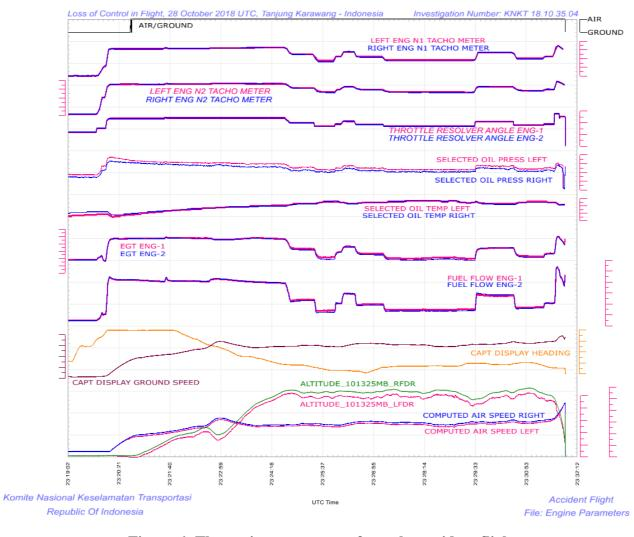
Figure 6: The engine parameters from the accident flight
