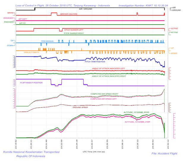
Figure 5: The significant parameters from the accident flight
