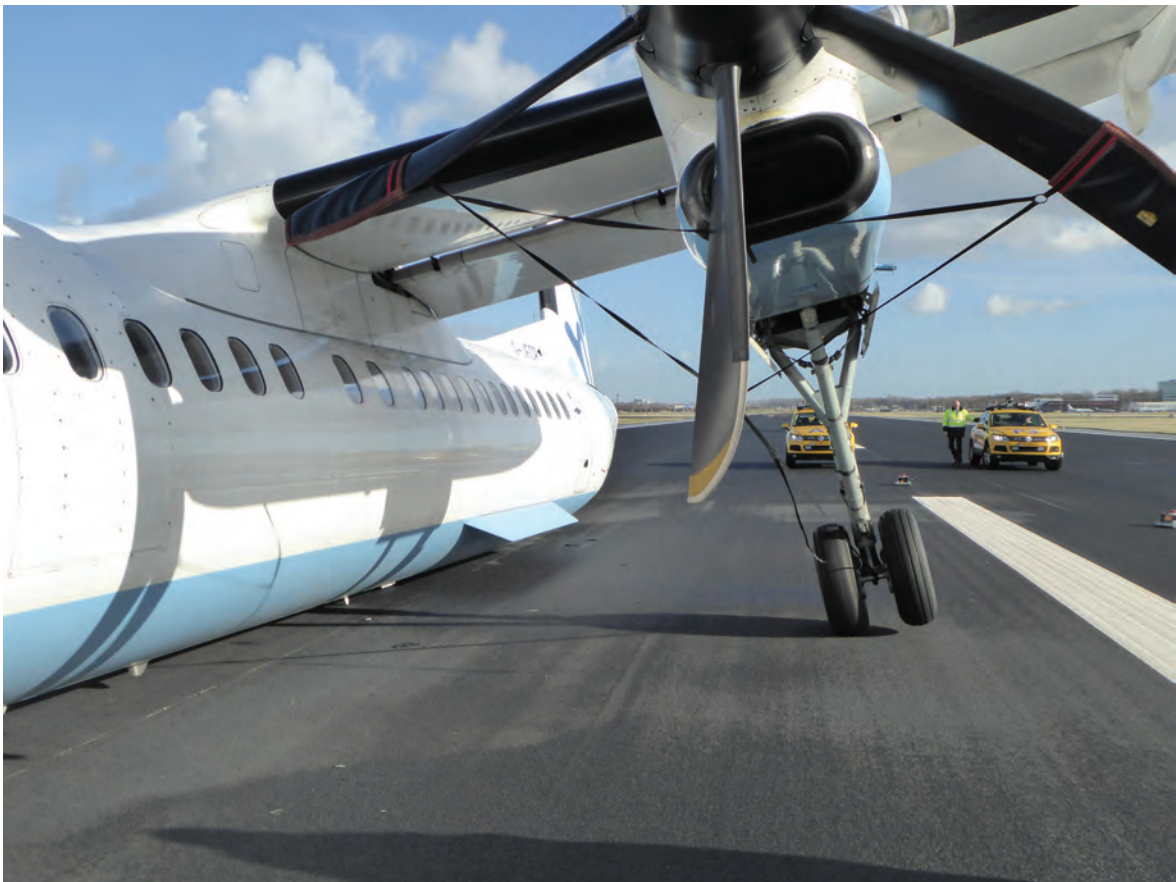
Figure 5: left-hand nacelle and MLG after occurrence. (source: Dutch Safety Board)
