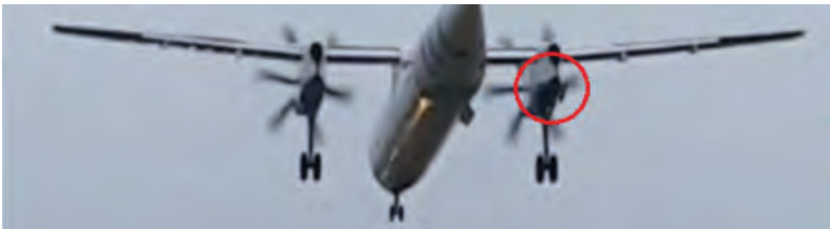
Figure 2: moment just before landing, viewed from rear, showing aft doors open on RH MLG. (still of video)
