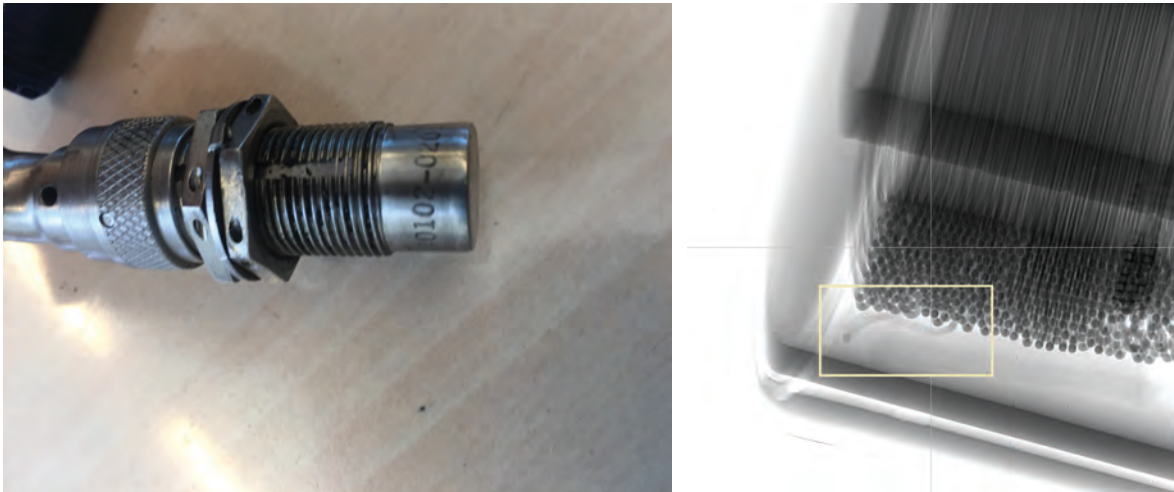
Figure 18: proximity sensor, and x-ray of sensor showing irregularity in loom.
