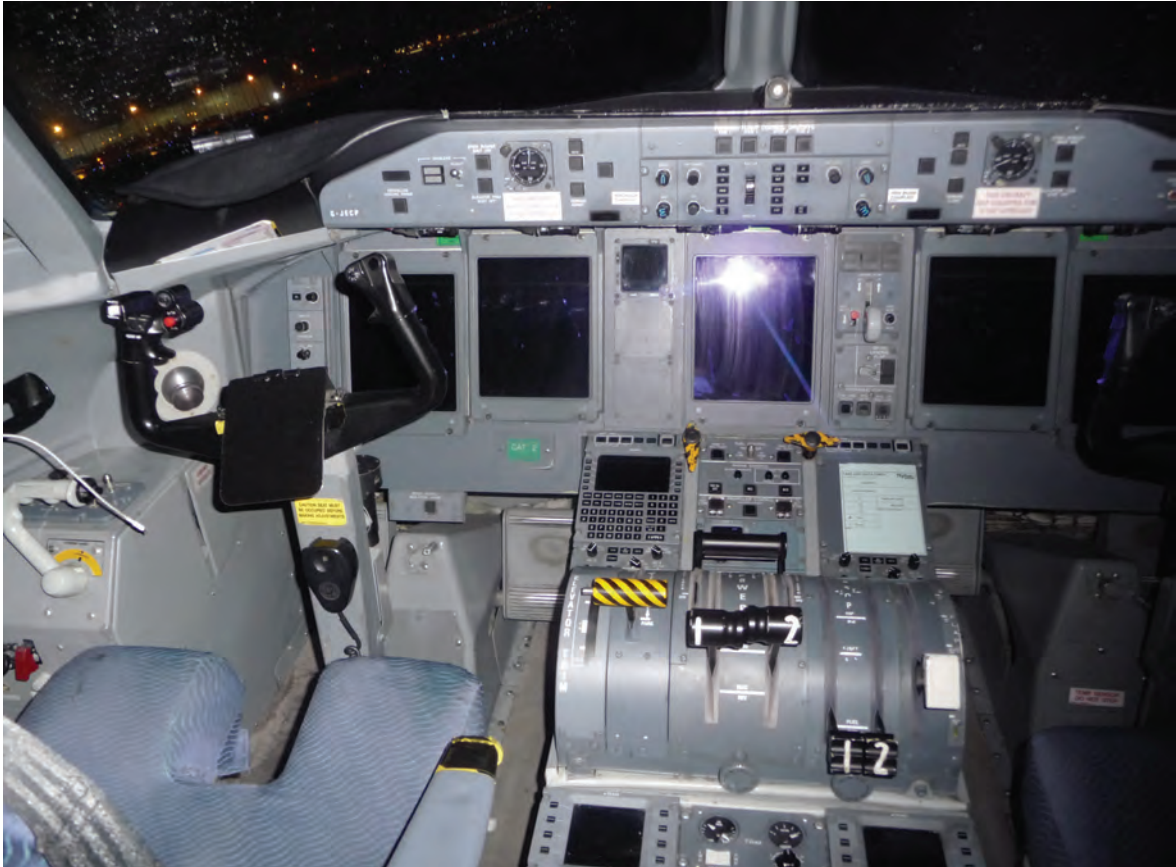
Figure 12: landing gear control panel in flight deck position. (source: DSB)
