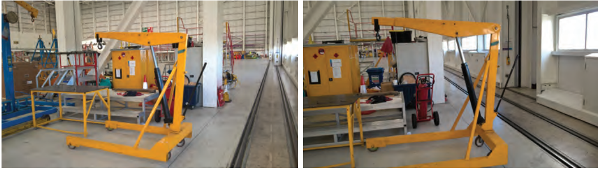
Figure 7: example of manual cranes used to lift the main wheels from the ground when replacing the brace assembly. (source: maintenance facility)
