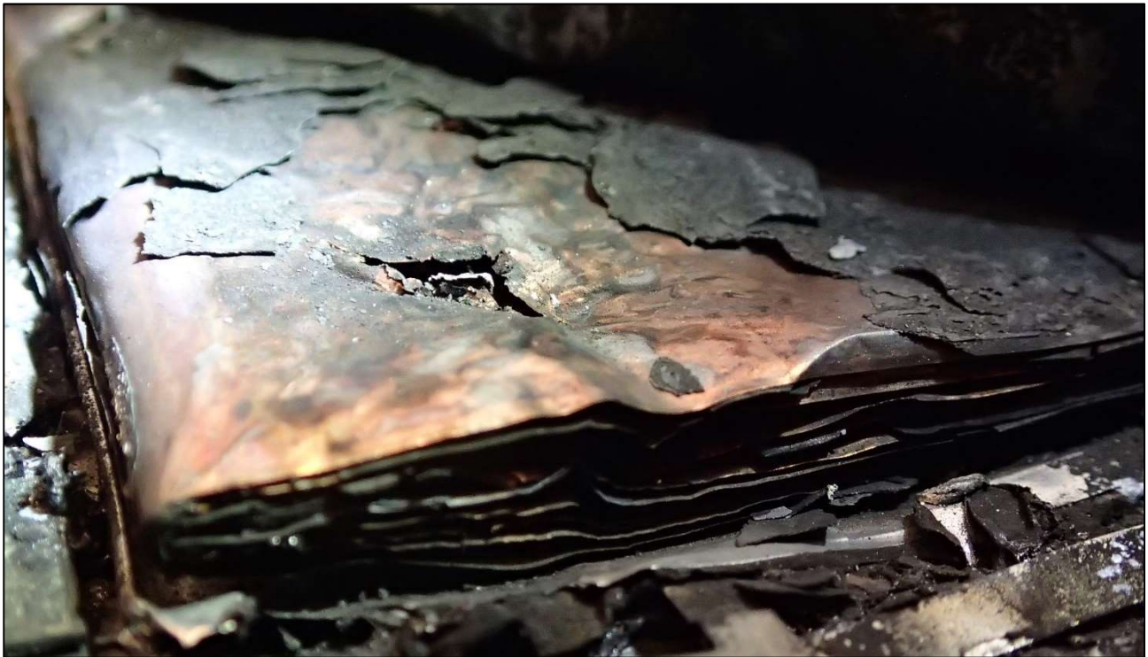
Figure 5. Close-up of the laptop battery's damages (Photo: SIA)
