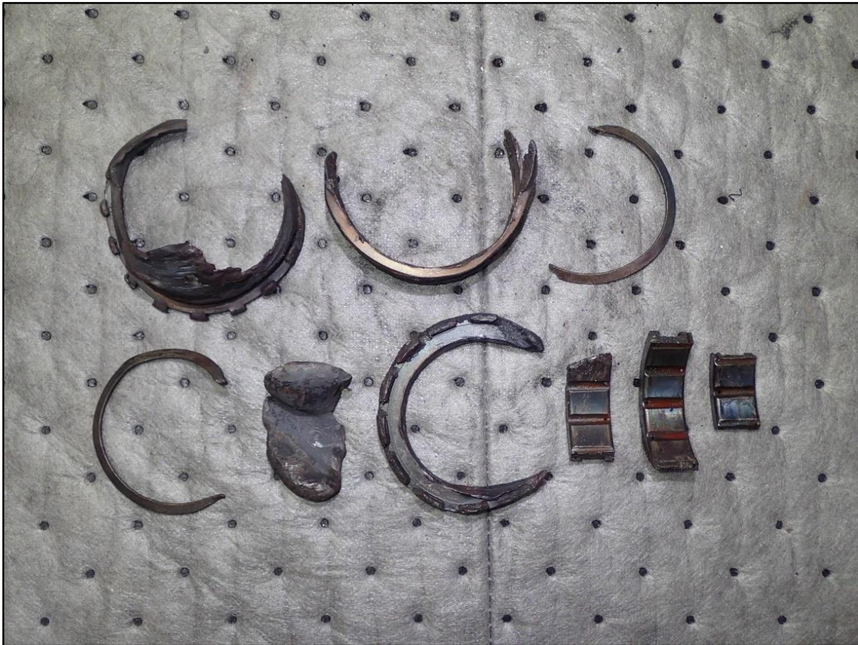
Remaining of no. 2 roller bearing, no. 2 bearing airseal, and no. 2 bearing nuts
