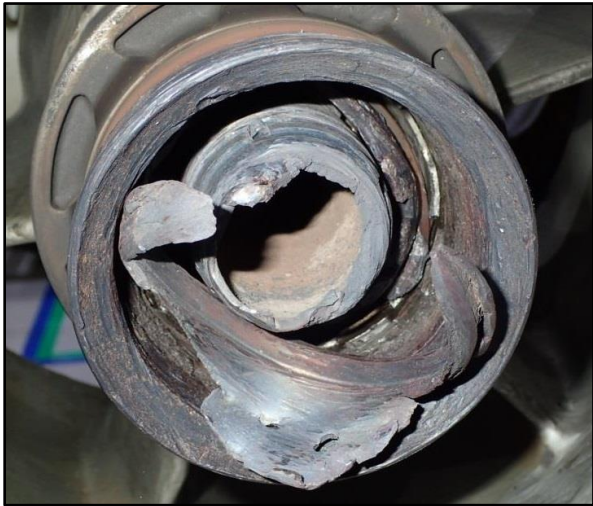
No. 2 bearing housing distress
