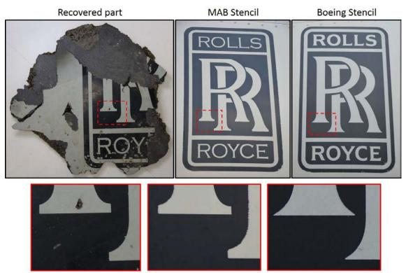
Note the thickness of the "ROYCE" lettering and the serif geometry on the main 'R's (enlarged for ease of comparison). Source: Malaysian MOT / ATSB
