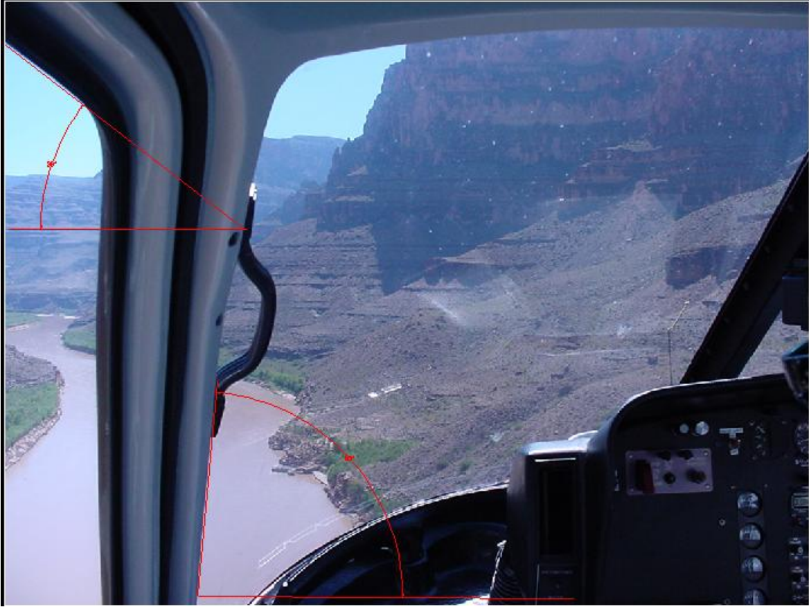
Figure 5. View of the level attitude reference angles for the accident helicopter.
